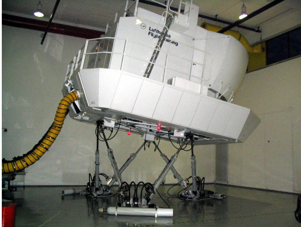
A hexapod non-orthogonal 6-strut mount (Image credit: Ethan Arnold )
